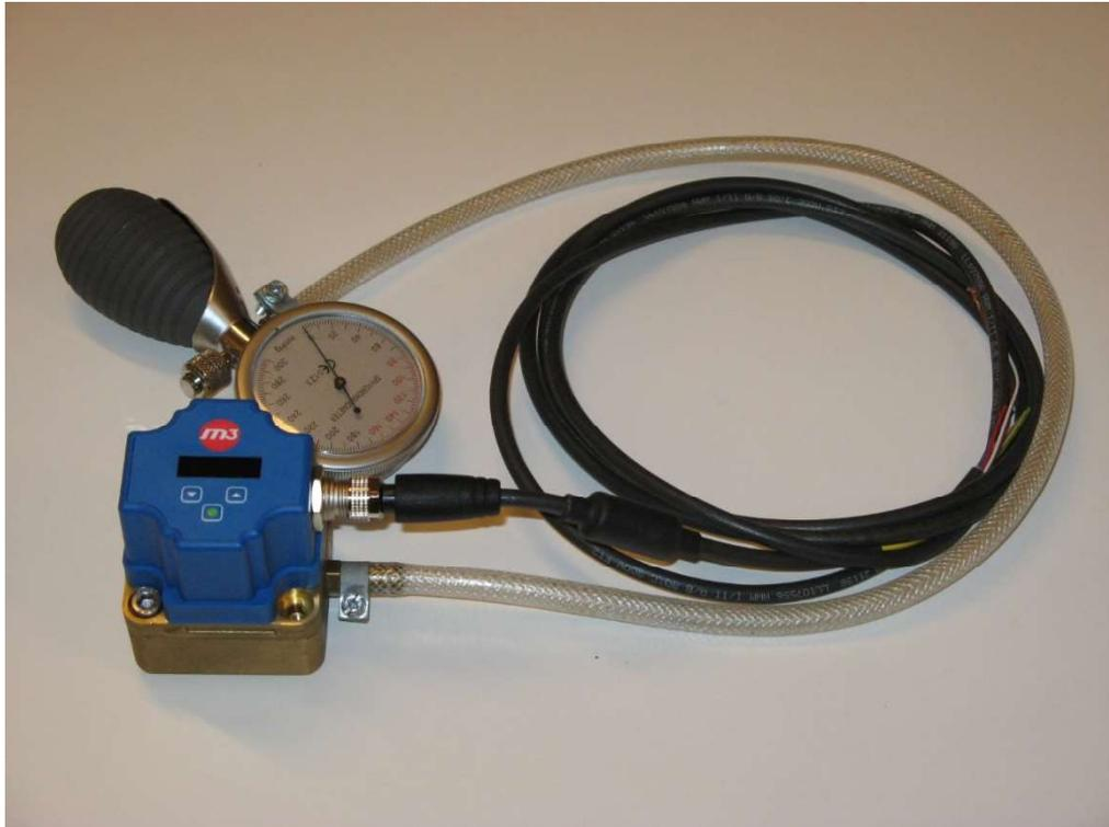
Photo 2.1.1 M3 Display with air pump
