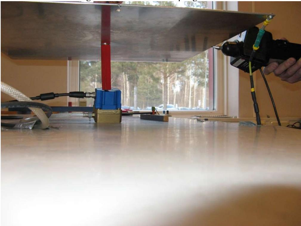
Photo 4.1.4 Test setup regarding immunity to electrostatic discharges.
