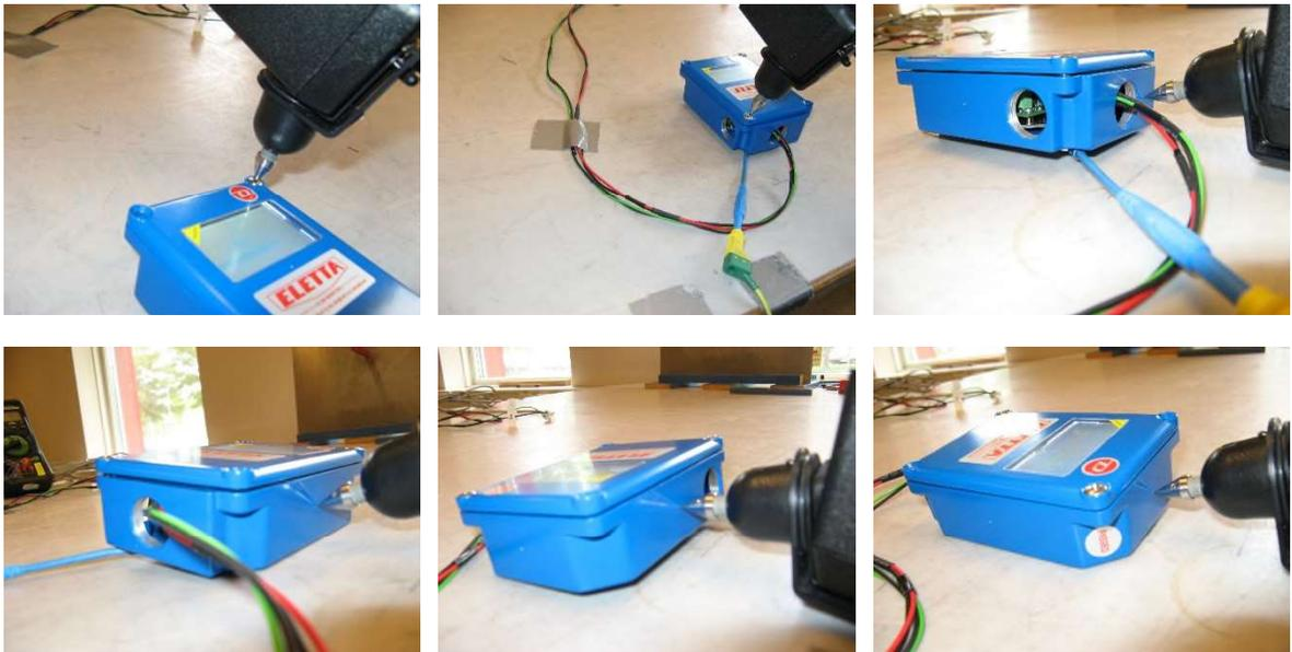
Photo 4.1.7 Test setup regarding immunity to electrostatic discharges. Test points for direct contact discharges.
