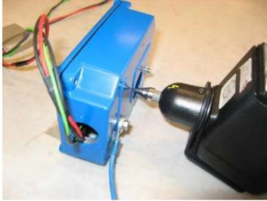
Photo 4.1.8 Test setup regarding immunity to electrostatic discharges.
