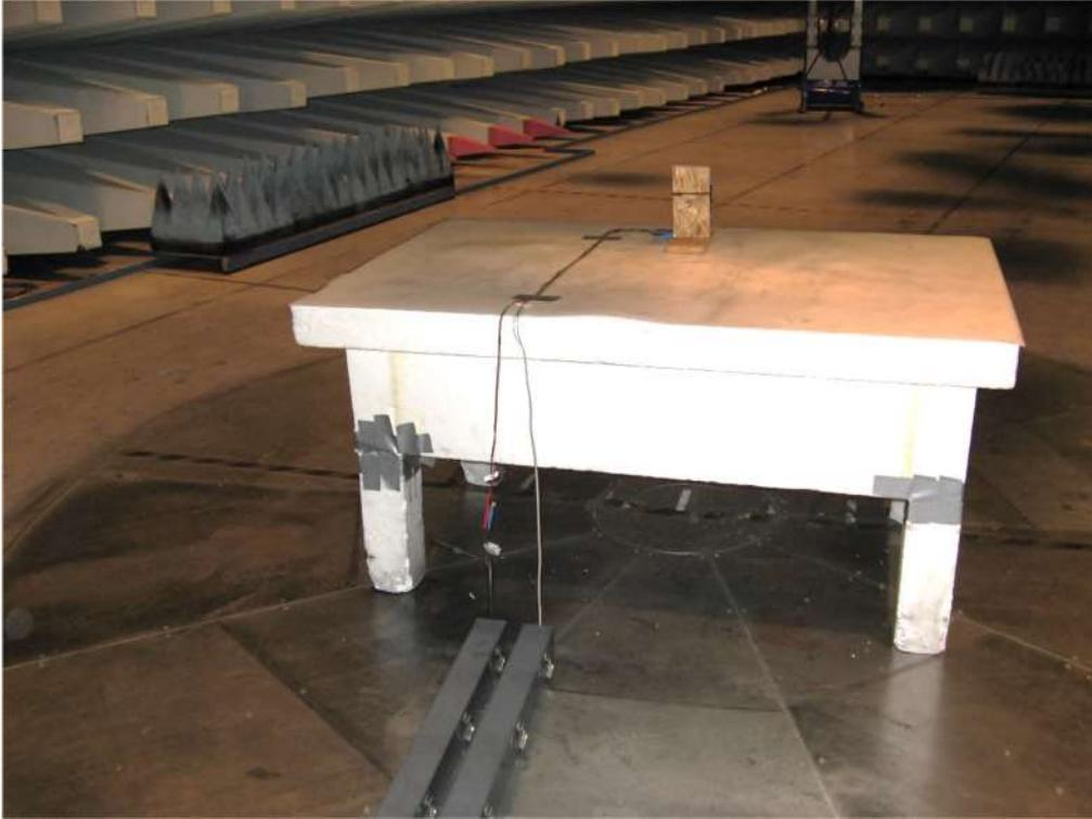
Photo 4.6.3 Test setup regarding measurement of radio frequency electromagnetic field. Rear view.
