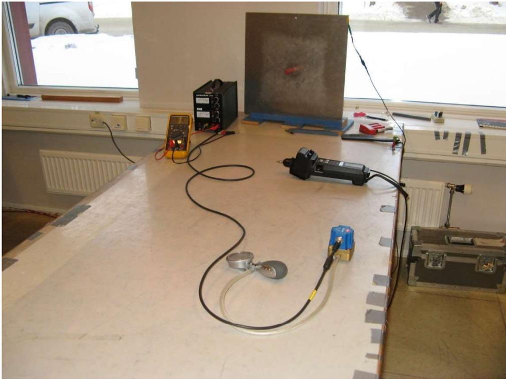
Photo 4.1.1 Test setup regarding immunity to electrostatic discharges.
