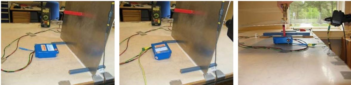
Photo 4.1.5 Test setup regarding immunity to electrostatic discharges.
