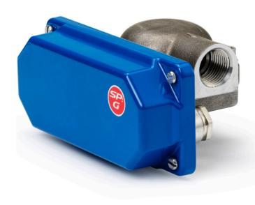
Our flow switch SP-G is designed to fit small flow and line sizes. It works on the principle of variable flow area where the alarm switch point can be set at a very low flow and still the switch is capable of handling large flows without creating a large pressure drop.
