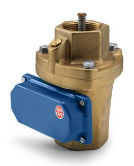
SP-GA Flow Switch is designed to give an initial alarm at a very low flow and still be capable of allowing a high full liquid flow passing through when pumps or valves are activated by the micro switch. The function is based on fluid flow activation only and threfore it is not affected by changes in static pressure.
