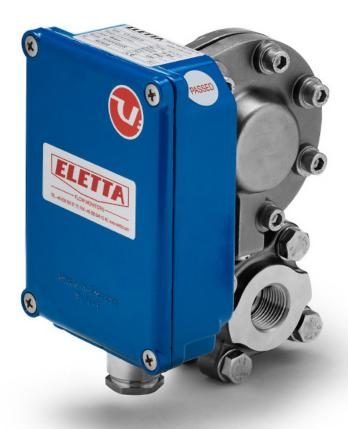
The V-series is a very robust and reliable flow monitor for harsh and dusty industrial environment. The V series has one micro switch setpoint, that is independently adjustable within the measuring range and can be set for high or low flow alarms for example to protect expensive equipment in various piping systems.
