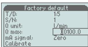
Scroll down to “Q max” and press the “M” button and the input box will light up. Set the right value according to the new orifice
