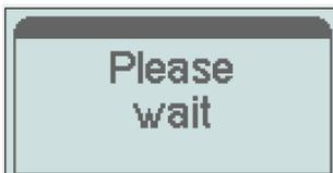
The adjusting of the calibration takes some seconds and during this time you need to keep the flow stable.
