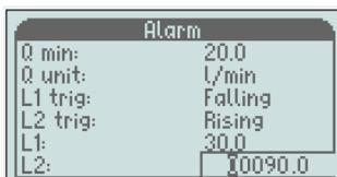
**Note!** It is not possible to set the alarm outside the flow range (Q min/Q max) Also the hysteresis effects on the alarm settings. L1 cannot be set higher than Q max - "Hyst1", and L2 can't be set lower than Q min + "Hyst2".
