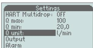
Scroll down to "Q unit" with the "-" button and press "M", to move to the right and now you can change the displayed units with "+/-" and choose between:
