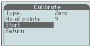
Scroll down to "Start" with "-" and press the "M" button
