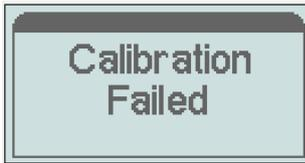
If the calibration Failed, the display goes back to the “Calibrate menu”, and you have to do a new calibration by starting from the beginning of the calibration procedure.
