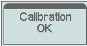
After the last calibration point you get a confirmation whether the calibration was “OK” or “Failed”.
