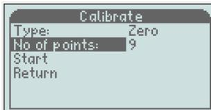
Scroll to "No of points" and choose how many calibration points you want to set. From factory, Turn down 1:5 is calibrated at 9 points and Turn down 1:2 at 6 points (D5 and D2 respectively).
