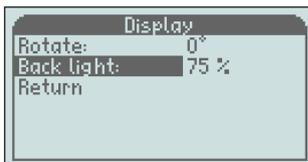
The backlight can be changed in 5 different levels, Off, 25, 50, 75 and 100%
