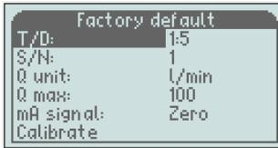
To leave the menu, scroll down to “Return” and press the “M” button, or hold the “C” button during 2 sec.
