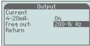
To activate the output, scroll down to "Freq out" and press the "M" button.
