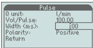
To set the pulse width, you change the figure by figure with "+/-" and confirm with "M". Next figure will be highlighted and you repeat until you get your desired value.
