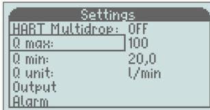
When there is only a frame around the word, you can't change anything as this is only an information field. In the example to the left you can see the actual flow range, Q max and Q min
