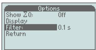
This filter will slow down the response time for the output signal and the displayed flow value.
