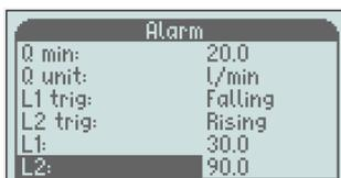
Scroll down with the "-" button to L1 or L2 and press the "M" button and the input box will light up.
