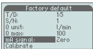
The output signal can be set in two different ways; “Zero” (zero-based) means that 4-20 mA represent 0-100% of Q max. This is most common and the factory default.
