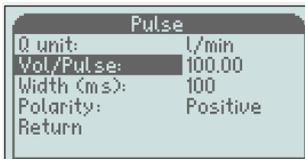
Scroll down with the "-" button to "Vol/Pulse" and press the "M" button and the input box will light up.
