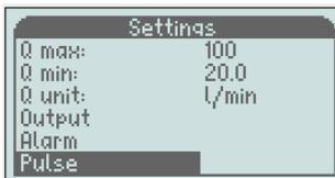
To change the pulse settings, scroll down with the "-" button to "Pulse" and press the "M" button
