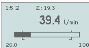
The totalizer works as long as the flow is within the flow range. If the flow should go outside the range or there is a power failure, the totalizer goes back to “Off” and also disappear from the display. If you want to go back to totalizing mode, you need to reactivate it.
