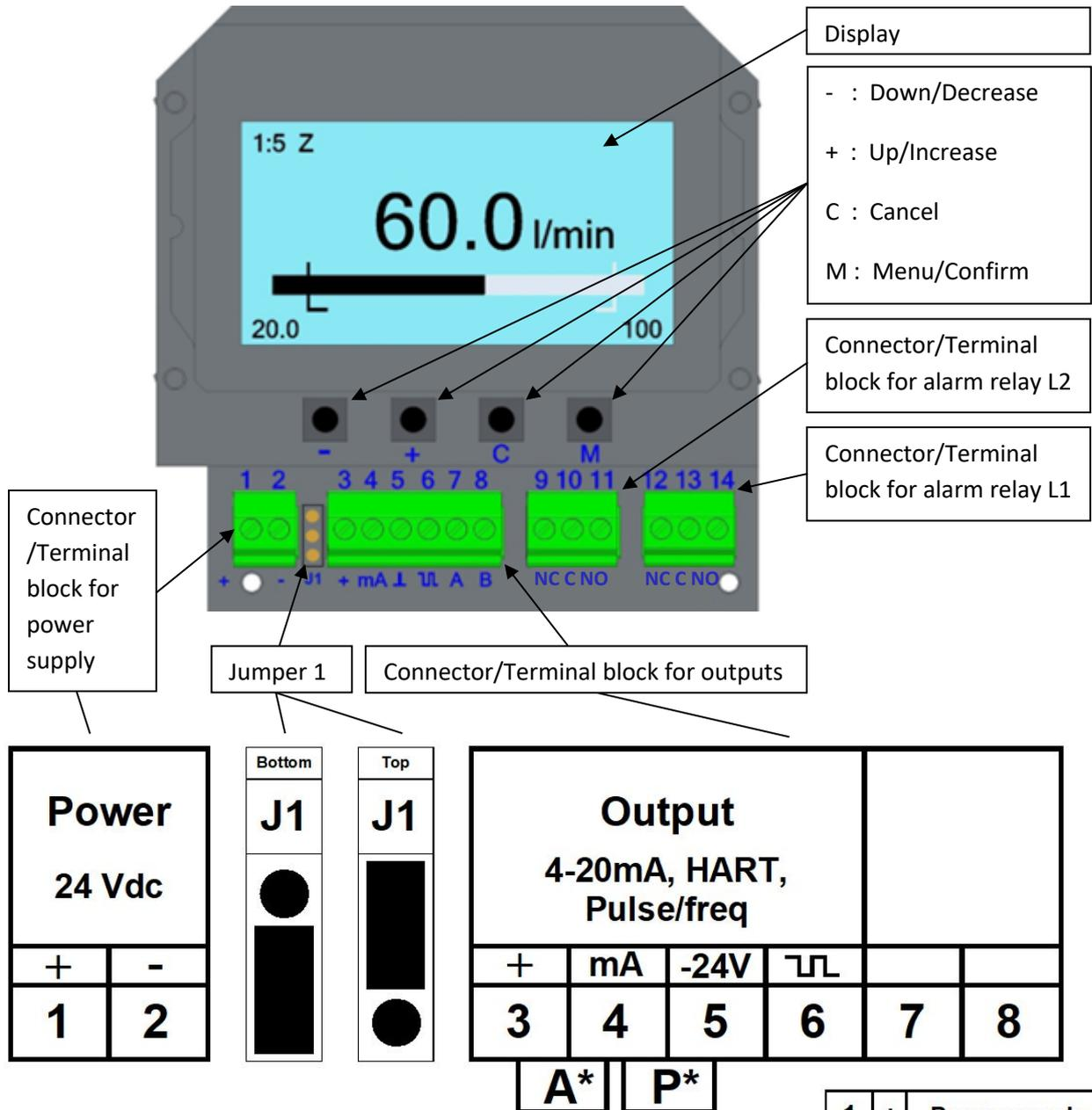
**Note!** The jumper fitting only affects the Pulse/freq. output.
