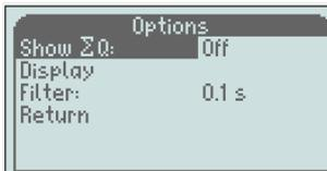
To activate the totalizer; when “Show  $\Sigma Q$ ” is highlighted press “M” to move to the right.
