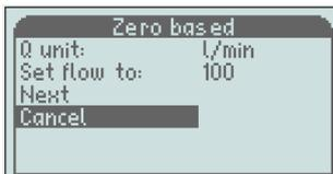
If you have come this far by mistake, you can interrupt the calibration without causing any changes here or you can go on with the calibration by adjusting a stable flow through your reference meter matching the value on the display "Set flow to".
