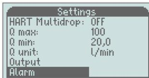
To change the alarm settings, scroll down with the "-" button to "Alarm" and press the "M" button
