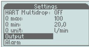
Scroll down to "Output" with the "-" button and press the "M" button.
