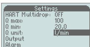
To leave this menu, scroll down to "Return" and press "M", or hold "C" button during 2 sec. "Return" takes you back one step in the menu, the "C" button takes you back directly to the operating mode.
