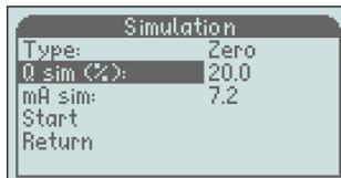
To activate the simulation, scroll down in the "Main menu" until "Simulation" will be highlighted and press the "M" button. Scroll down to "Q sim" or "mA sim" and press the "M" button, and the input box will light up.
