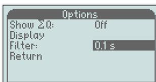
To change the filter value, scroll down in the "Options" menu until "Filter" will be highlighted. Then press "M" and the input box will light up.
