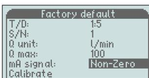
To change, scroll down to “mA signal” and press the “M” button to move to the right, and then change by using “-/+” and confirm with the “M” button
