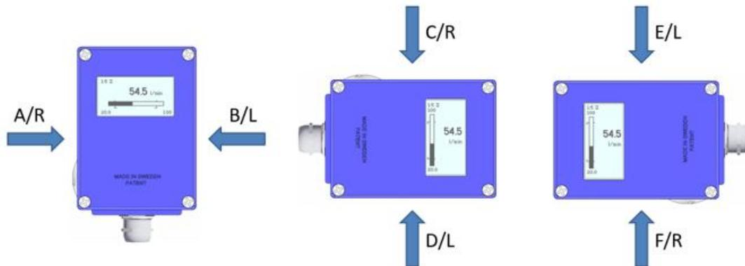
It is very important that the Flow Monitor is mounted in the correct flow direction as the function of the Flow Monitor otherwise will be prevented. The flow direction arrow that is located on the Pipe Section denotes the flow direction which needs to correspond with the flow direction in the system.
