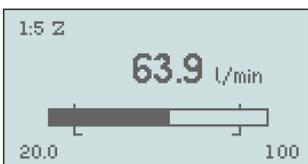
The flow value shows constantly as long as the flow is within the flow range. Within 2% below Q min and above Q max, the value will flash before it goes over to show “Low flow” or “High flow”
