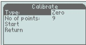
Chose "Type"; Zero or Non-zero, by pressing the "M" button and use "-/+ " to change and confirm with the "M" button.
