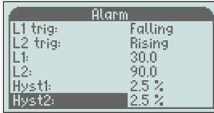
The hysteresis is necessary to avoid the alarm to ripple (go on and off) when the flow is close to the set point.
