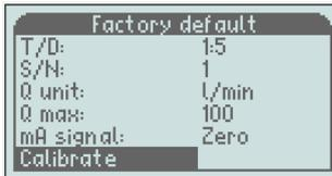
**Note! The Flow Meter is already calibrated from factory and it shall normally not be necessary to recalibrate.**
