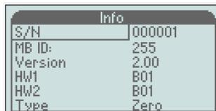
This menu will give you information about the version of software and hardware and also the type of output signal i.e. Zero-based or Non-Zero based.
