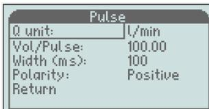
**Note!** The pulse needs to be activated in the "Output" menu for the pulse to work.
