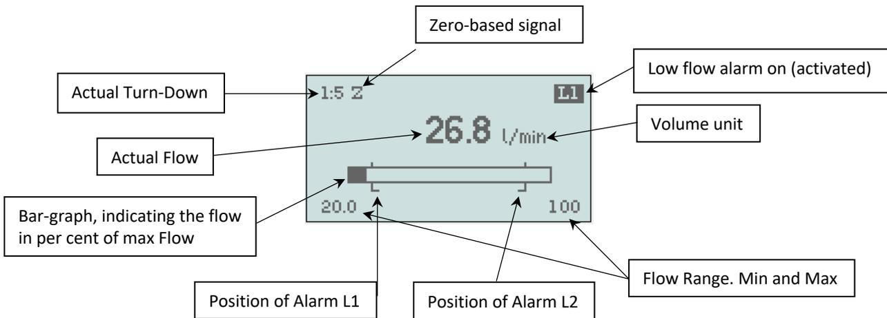
When you connect the power supply, the display lightens up, “Low flow” and “L1” will flash (if you don’t have any flow in process pipe).
