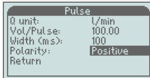
Scroll down with the “-” button to “Polarity” and press the “M” button to set the polarity to positive or negative.
