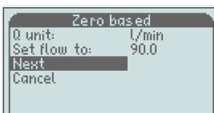
Next step in the calibration lights up and you can adjust to the flow the software ask for and press the "M" button to confirm.
