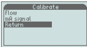
To leave this menu, scroll down to “Return” and press “M”, or hold “C” button during 2 sec. “Return” takes you back one step in the menu, the “C” button takes you back directly to the operating mode.
