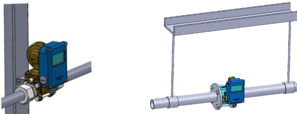
If your piping system still suffers from vibrations, we recommend a separate mounting of the Pipe Section and Control Unit. See chapter 2.5.
