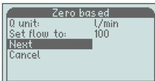
Move with "+" so "Next" will be highlighted and press the "M" button to confirm
