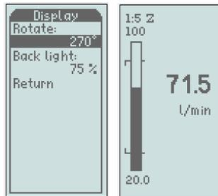
To leave this menu, scroll down to "Return" and press "M", or hold "C" button during 2 sec. "Return" takes you back one step in the menu, the "C" button takes you back directly to the operating mode.
