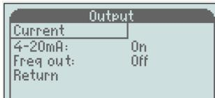
In this menu you can activate the frequency output. It gives a frequency of 200 to 1000 Hz or pulse.
