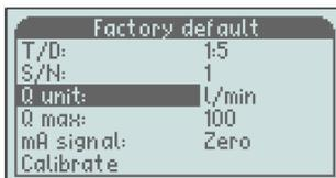
Scroll down to “Q unit” and press the “M” button to move to the right. Set the right unit for the new orifice by using “-/+”, and confirm with the “M” button.
