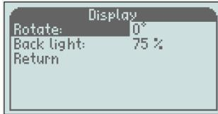
To change the orientation, scroll down to "Display" and press "M" and when "Rotate" is highlighted press "M" to move to the right. Use "+" or "-" to rotate to the angle you want, and confirm with "M".
