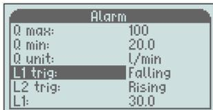
Scroll down with the "-" button to L1 trig or L2 trig and press the "M" button to set L1 or L2 to falling or rising. L1 is set to falling and L2 is set to rising by default from the factory.
