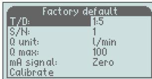
T/D: show you the actual flow turn down, in this case 1:5 (Q min is five times less than Q max).
