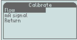
Scroll down to "calibrate" and press the "M" button and when "Flow" is highlighted press the "M" button once more.
