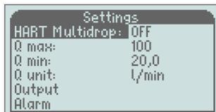
HART Multidrop mode restricts the output current to 4mA, for use when multiple HART instruments are connected to a singular signal loop. To activate HART Multidrop mode; when "HART Multidrop" is highlighted press "M" to move to the right.
