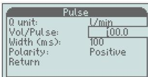
To set the pulse per unit volume, you change the figure by figure with "+/-" and confirm with "M". Next figure will be highlighted and you repeat until you get your desired value.
