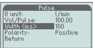
Scroll down with the "-" button to "Width (ms)" and press the "M" button and the input box will light up.
