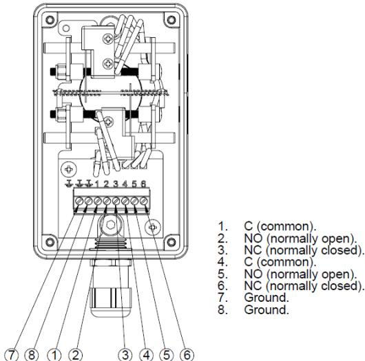
Figure 5, Wiring diagram
