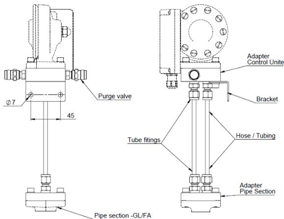
Figure 2, Separate mounting GL/FA
