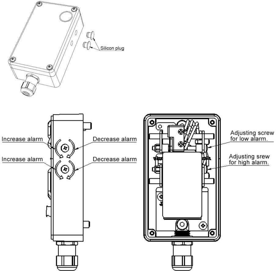
**Adjusting of high/low flow alarm for V2/V25**
