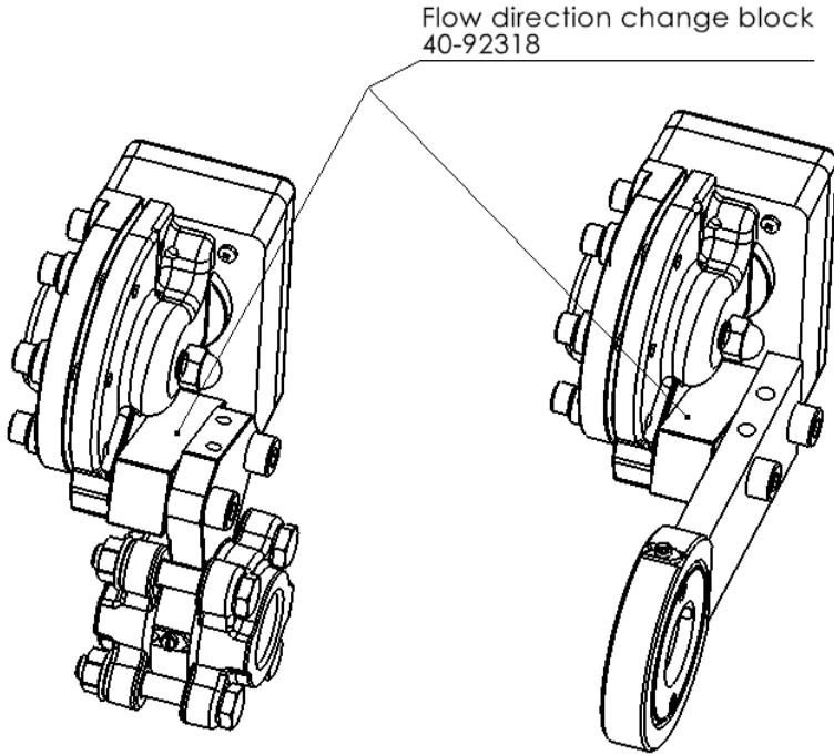
*Figure 7, Flow direction selector*
