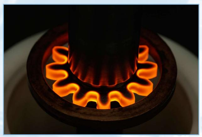
Contour hardening of gears with EFD Induction's patented multi frequency concept. The surface of the gear is heated to 1000° C within a few seconds to achieve the correct hardening depth.
