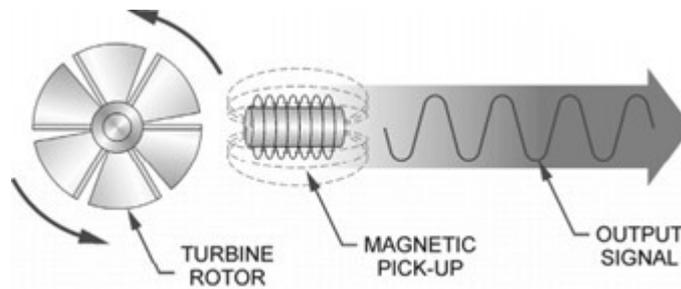
For better flow measuring results, Turbine flow meter are recommended to use for liquid flow measurement having viscosity less than 10 Cst. However here the grinding aid chemical's viscosity is around 20 Cst so it is not suitable.
