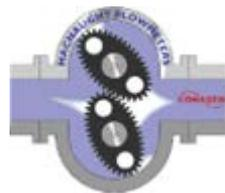
In existing chemical dispensing skid, Mag meters were replaced by an Oval Gear type flow meter of 10mm size, but that did not work either.
