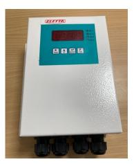
All M series units are supplied with a panel or wall mounted LED displays, that takes in 230 VAC from the wall, converts it to provide 24 VDC to the M Series and takes back its 4-20mA output on the same loop for local display and totalization.
