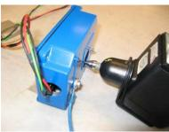
Photo 4.1.8 Test setup regarding immunity to electrostatic discharges.
