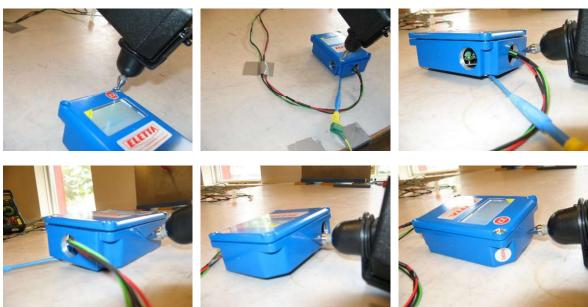
Photo 4.1.7 Test setup regarding immunity to electrostatic discharges.
