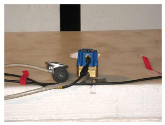
Photo 4.2.4 Test setup regarding immunity to radio frequency electromagnetic field. Left side (with cable inlet) exposed to the field.
