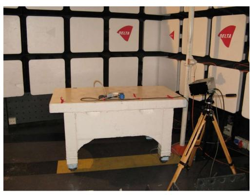
Photo 4.2.1 Test setup regarding immunity to radio frequency electromagnetic field for test between 80-1000 MHz.
