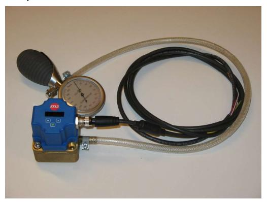
Photo 2.1.1 M3 Display with air pump
