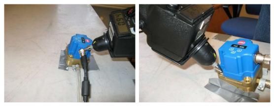
Photo 4.1.6 Test setup regarding immunity to electrostatic discharges. Sample of test points for direct contact discharges.
