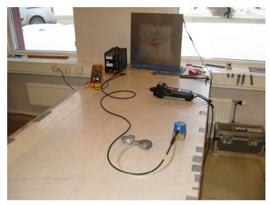
Photo 4.1.1 Test setup regarding immunity to electrostatic discharges.
