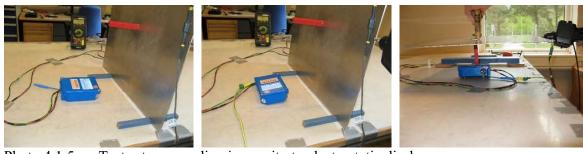
Photo 4.1.5 Test setup regarding immunity to electrostatic discharges.
