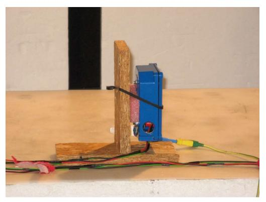
Photo 4.2.4 Test setup regarding immunity to radio frequency electromagnetic field. Left side exposed to the field.
