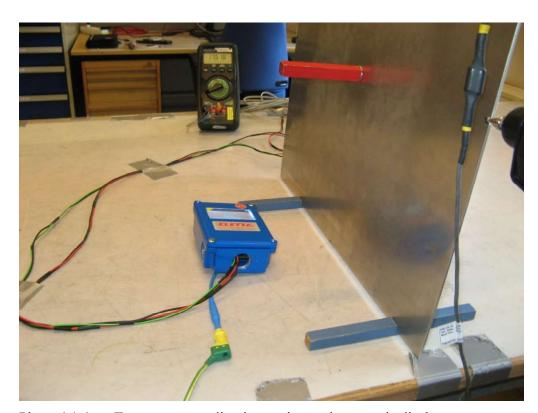
Photo 4.1.4 Test setup regarding immunity to electrostatic discharges. Discharges via VCP indirect coupling.
