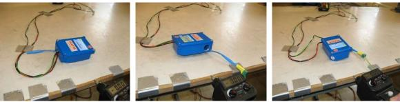
Photo 4.1.3 Test setup regarding immunity to electrostatic discharges.
