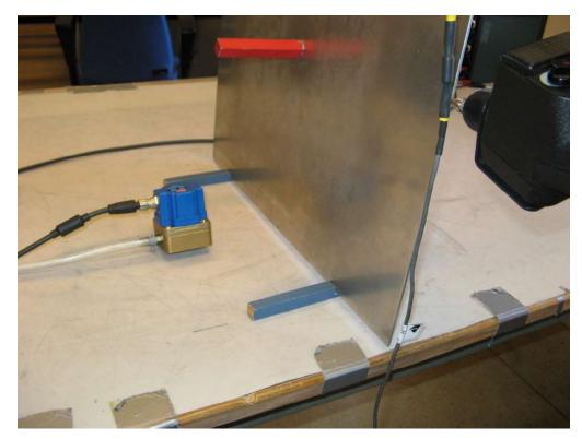
Photo 4.1.3 Test setup regarding immunity to electrostatic discharges.
