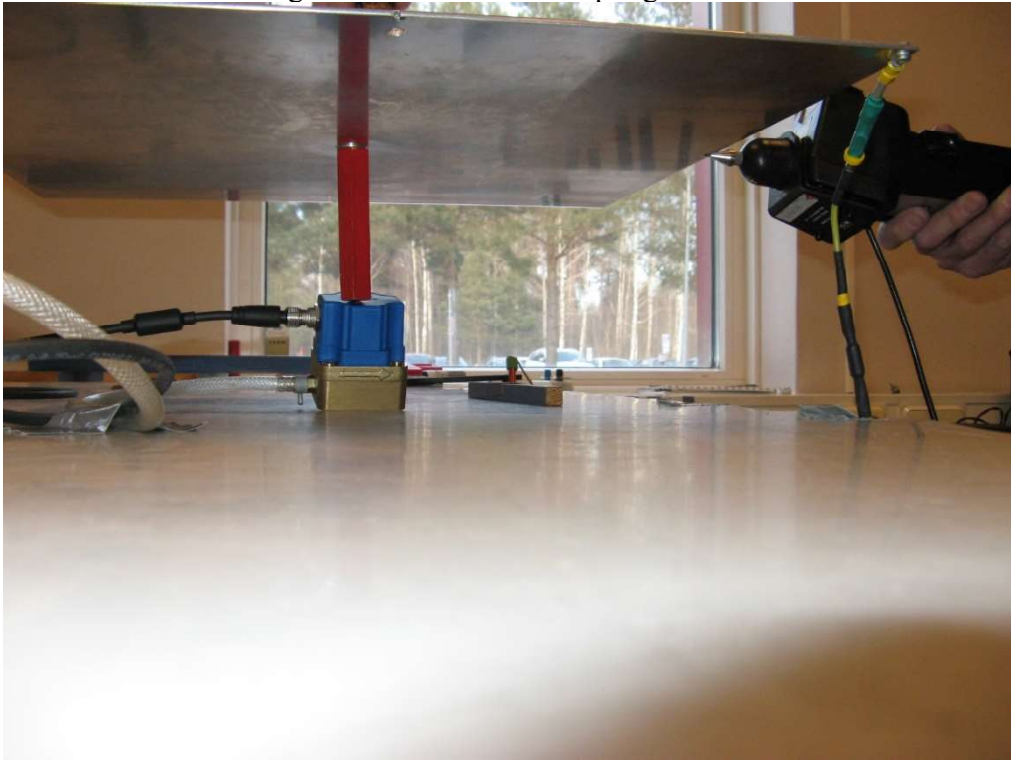
Photo 4.1.4 Test setup regarding immunity to electrostatic discharges. Discharges via VCP indirect coupling.
