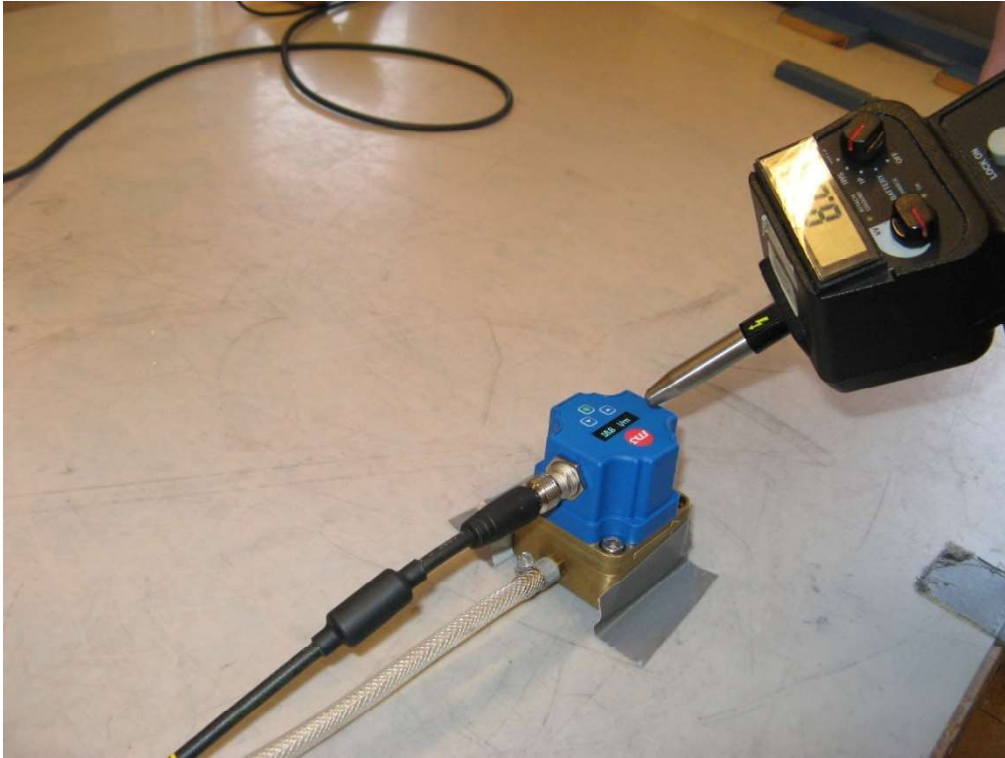
Photo 4.1.7 Test setup regarding immunity to direct air electrostatic discharges.
