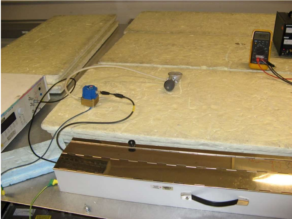
Photo 4.3.1 Test setup regarding immunity to fast transients on power + signal port. Test object grounded.
