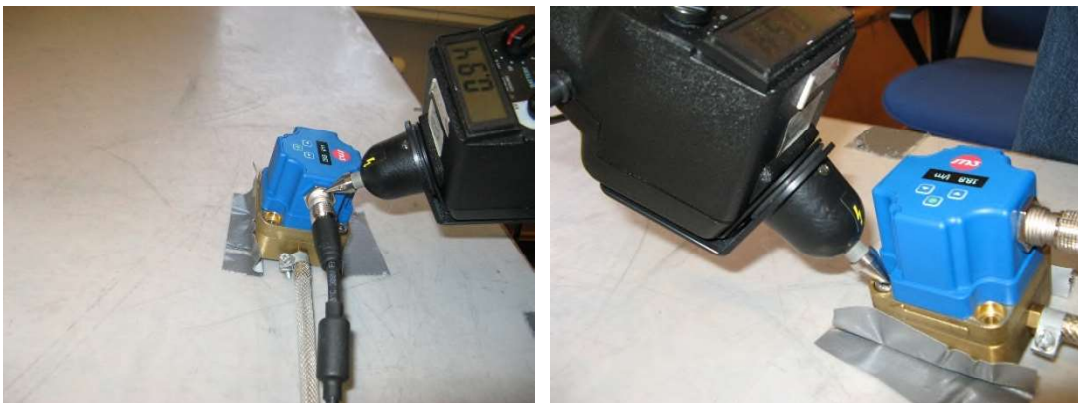
Photo 4.1.6 Test setup regarding immunity to electrostatic discharges. Sample of test points for direct contact discharges.
