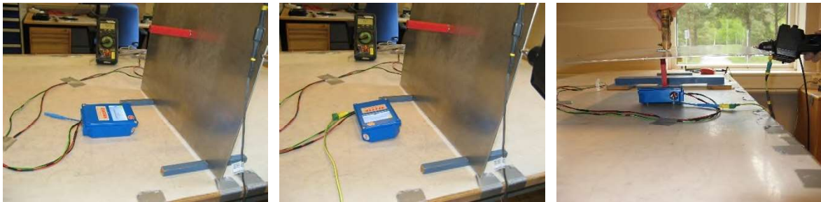
Photo 4.1.5 Test setup regarding immunity to electrostatic discharges. Discharges via VCP indirect coupling.
