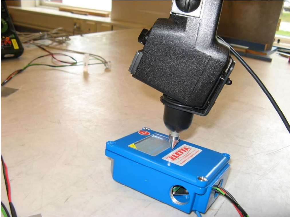
Photo 4.1.6 Test setup regarding immunity to direct contact electrostatic discharges.
