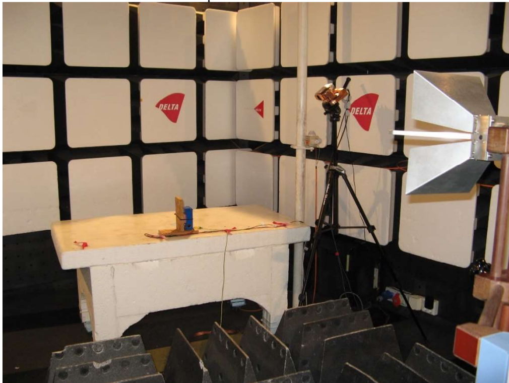
Photo 4.2.5 Test setup regarding immunity to radio frequency electromagnetic field for test above 1 GHz.
