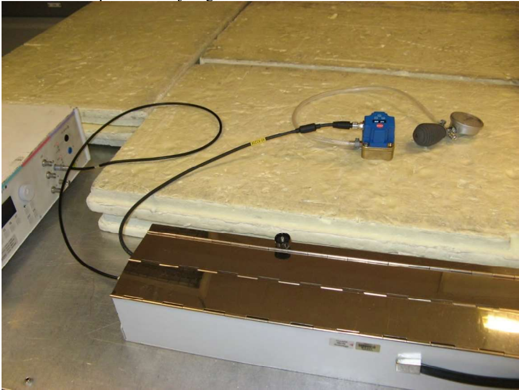
Photo 4.3.2 Test setup regarding immunity to fast transients on power + signal port. Test object not grounded.
