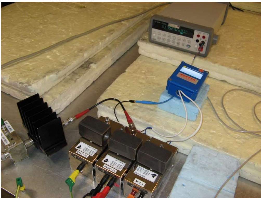
Photo 4.5.2 Test setup regarding immunity to conducted radio frequency disturbances on DC power port. Test object case grounded.
