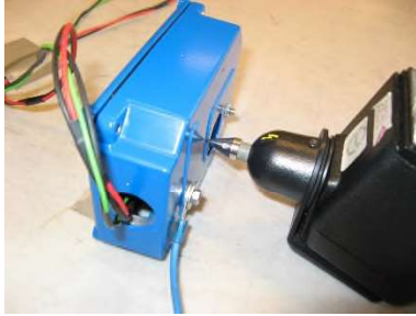
Photo 4.1.8 Test setup regarding immunity to electrostatic discharges. Test points for direct contact discharges.
