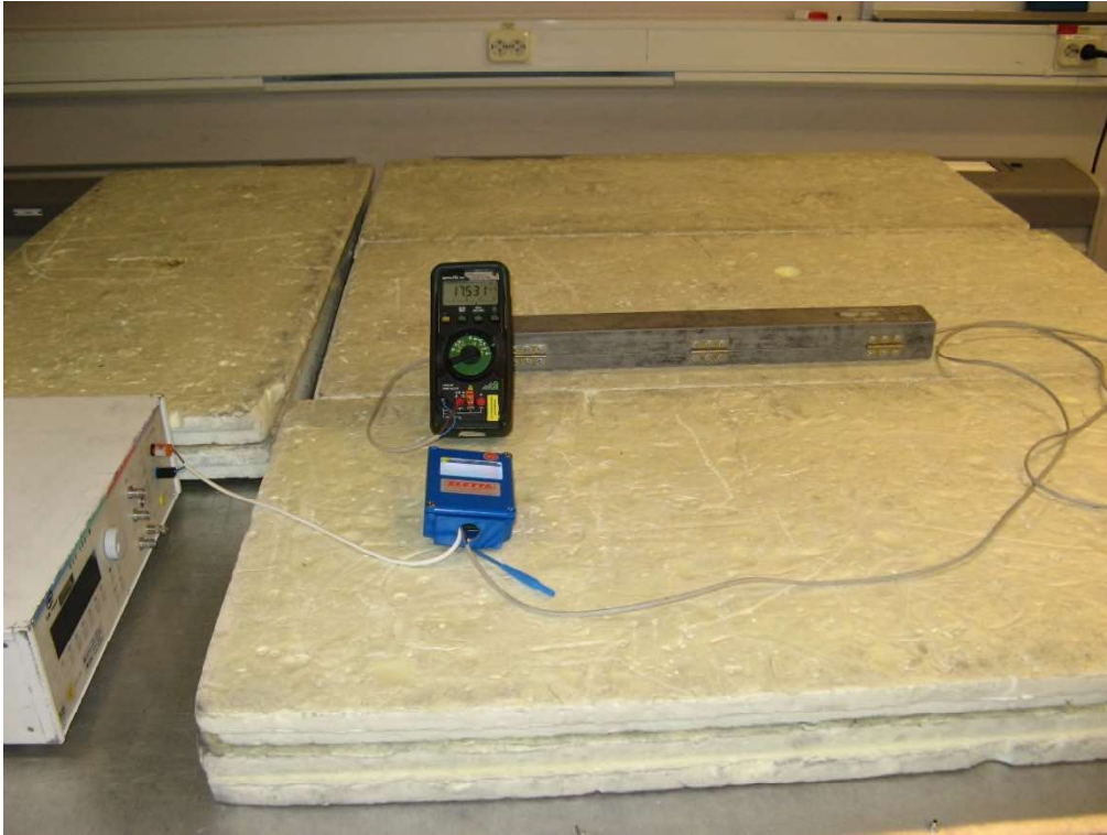
Photo 4.3.1 Test setup regarding immunity to fast transients.
