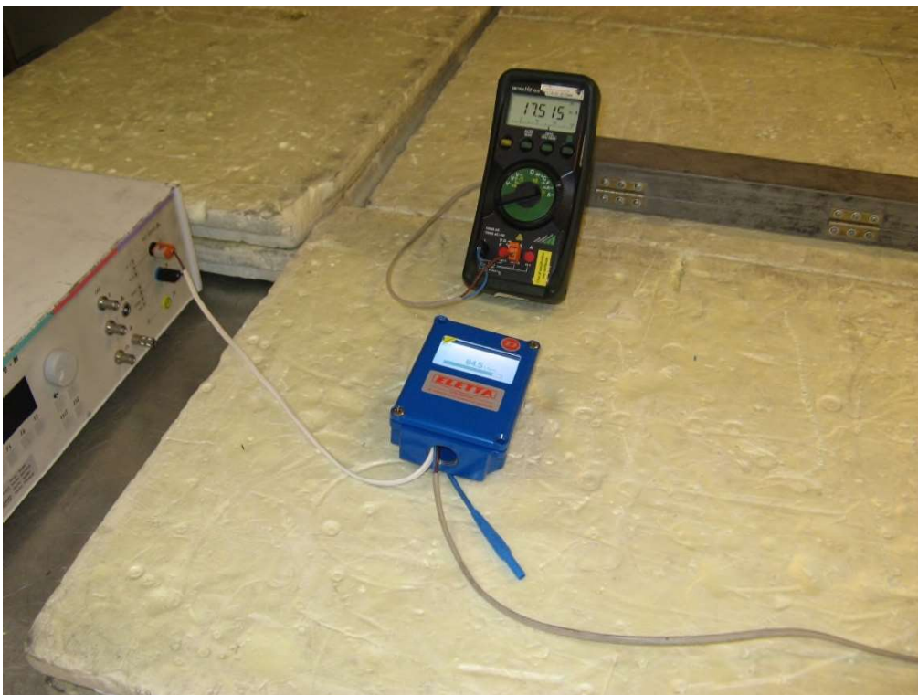
Photo 4.3.2 Test setup regarding immunity to fast transients on DC power port. Test object case not grounded.
