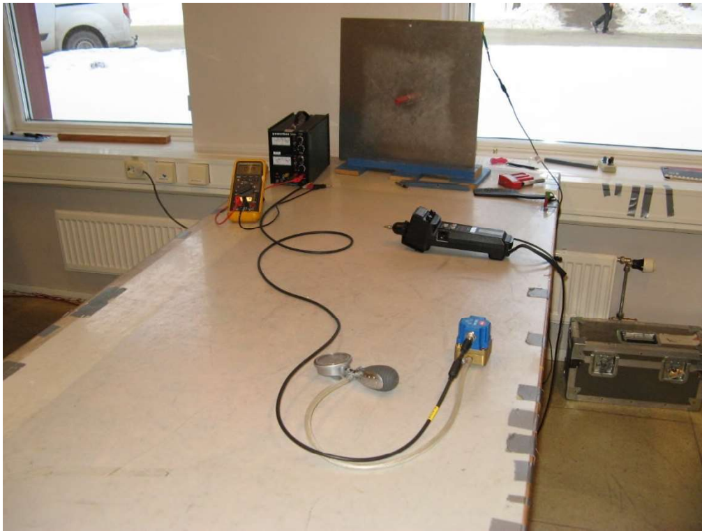
Photo 4.1.1 Test setup regarding immunity to electrostatic discharges.
