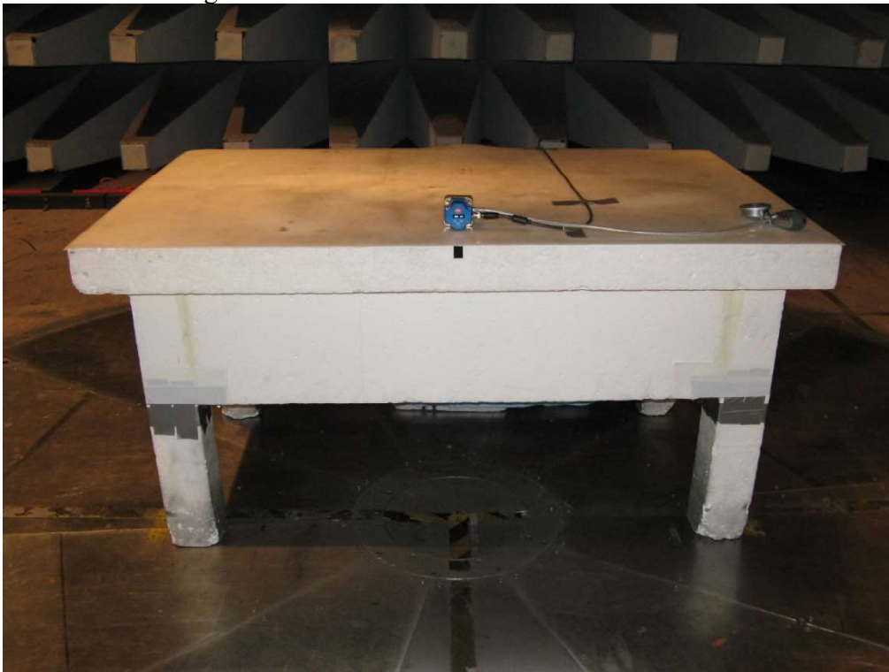
Photo 4.6.2 Test setup regarding measurement of radio frequency electromagnetic field. Front view.
