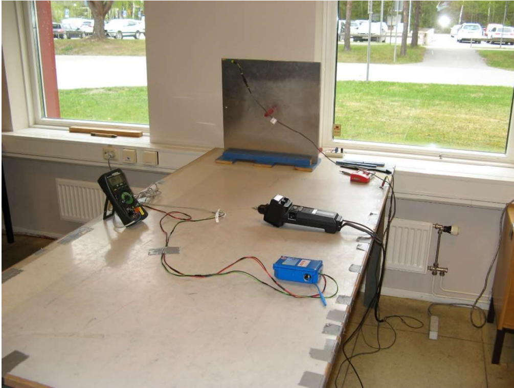
Photo 4.1.1 Test setup regarding immunity to electrostatic discharges.
