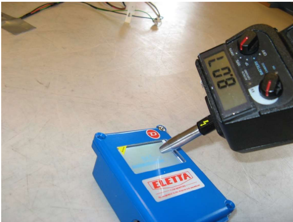
Photo 4.1.9 Test setup regarding immunity to direct air electrostatic discharges.
