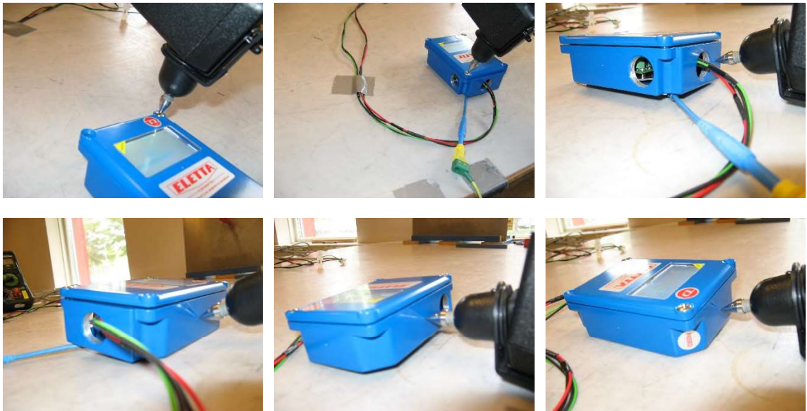
Photo 4.1.7 Test setup regarding immunity to electrostatic discharges. Test points for direct contact discharges.
