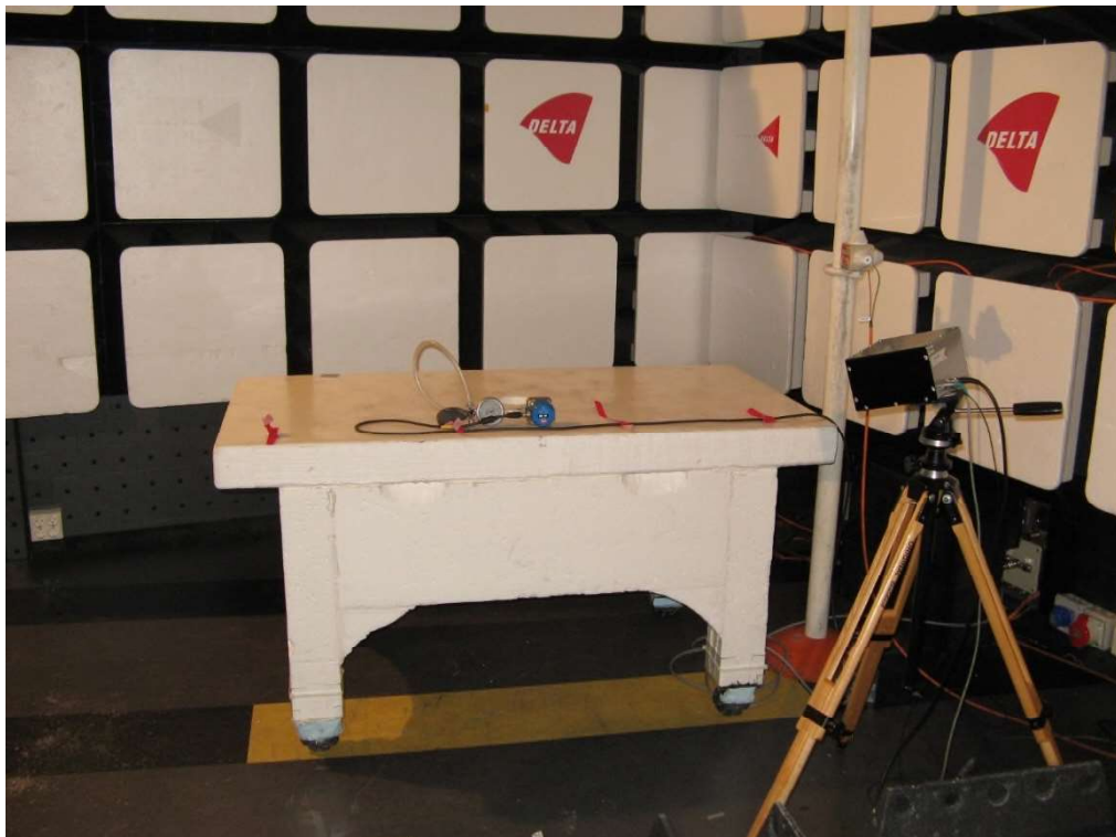
Photo 4.2.1 Test setup regarding immunity to radio frequency electromagnetic field for test between 80-1000 MHz.
