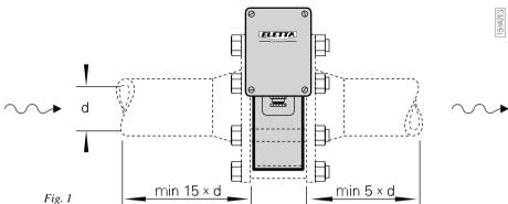
The reasons for this procedure is to achieve a stable flow profile inside the pipe and by doing so, get a true reading. Please be aware of the fact that it is practically impossible to predict when the flow is stable after disturbances in the piping, so this must serve as a guideline only.
