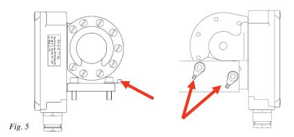
Ground terminals V-GL/FA Ex version for connection to pipe system
