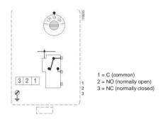
Fig. 6 The wiring diagram shows the switching function when the flow is zero or below the setpoint.
