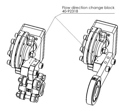
Figure 7, Flow direction selector
