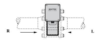
Figure 8, Flow direction alternatives
