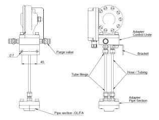
Figure 2, Separate mounting GL/FA
