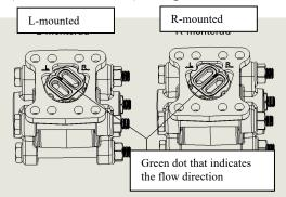
Figure 6, Flow direction selector
