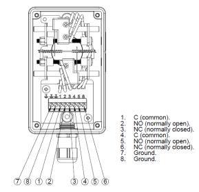
Figure 5, Wiring diagram
