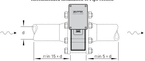
**Recommended installation of Pipe Section**
