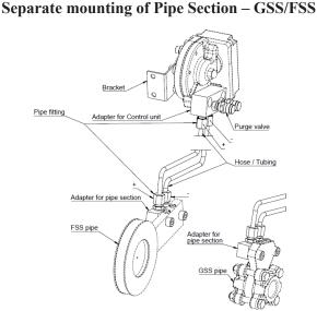
Figure 3, Separate mounting GSS/FSS
