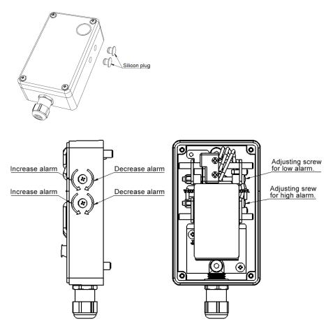
Adjusting of high/low flow alarm for V2/V25
